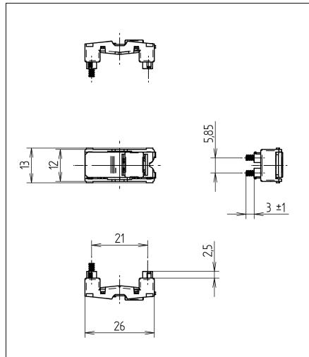
Custom designed for and in cooperation with a manufacturer of switches for household and similar fixed-electrical installations, this indicator light is an example of our design and production possibilities in the field of signalling devices using L.E.D.s as light source.
